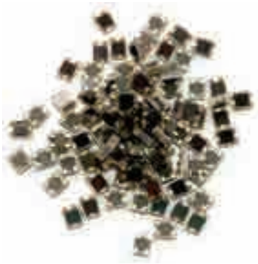
MicroRB sensors – 1 mm sensor in a robust molded leadframe package
